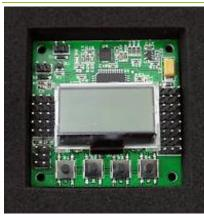
**STEP-1** Mount the FC on the frame with the LCD facing front and the buttons facing back. You can use the supplied antistatic foam container as a form of protective case for the Flight Controller on the craft.
