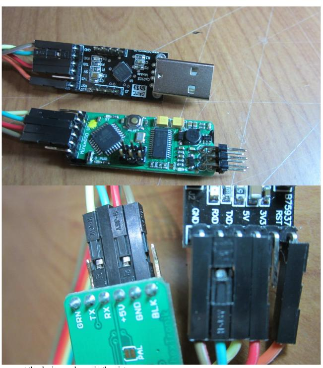
connect the device as shown in the picture find the serial port on start-control pannel-service-hardware- the avr isp device
