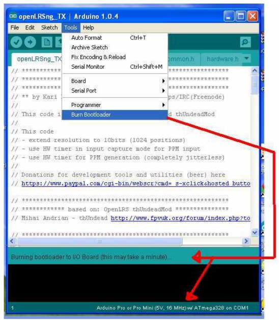
upload the bootloader and at the end disconnect the usbasp device you may see some kind of error but they are not important
