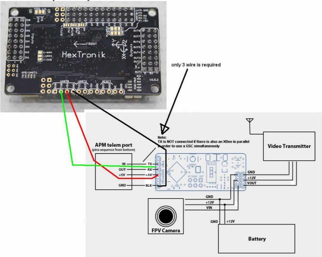
this is the right way ,the  $4^\circ$  wire is not necessary because the nimin osd need only listen the apm board
